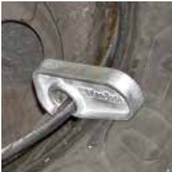
Newest Bead Holder - Made From Aluminum
