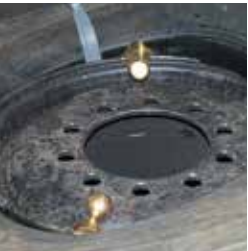
How to Properly Use Bead Holders #31710 on a 21L-24 Backhoe Tire and Wheel
