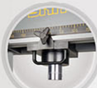
Scale & Sliding Cylinder with Handle and Rotatable Knob
