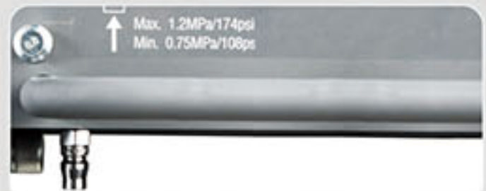
Pneumatic Power Set with Condensate Separator and Compressed Air Connections
