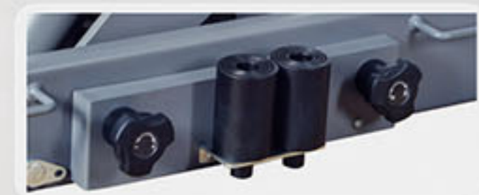
Two-hand lowering operation with automatic safety locking device and overload valve for optimum safety
